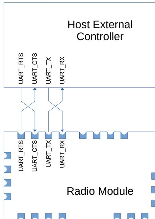
The serial UART communication needs to be configured with the correct parameters (baud rate, parity, start and stop bits) for successful communication.
