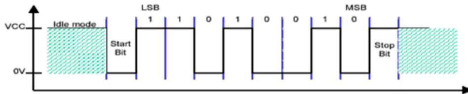
Figure 3: UART Data Packet (example 0x2B)
